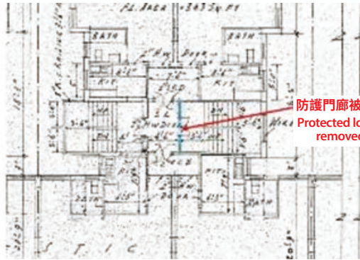
拆除逃生樓梯的防護門廊 Removal of protected lobbies of exit staircases
