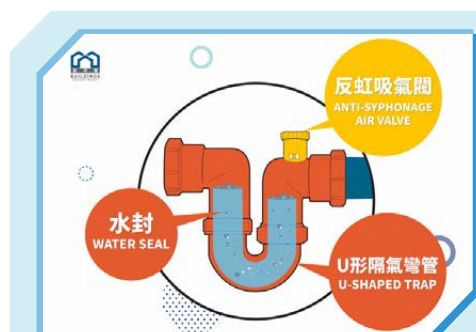
備有反虹吸氣閥的U形隔氣彎管 (安裝於地台去水口) U-shaped trap with anti-syphonage air valve (installed under floor drains)
