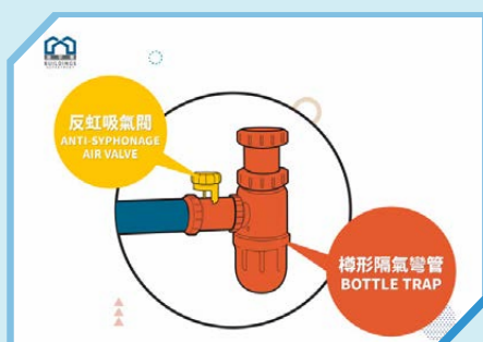
備有反虹吸氣閥的樽形隔氣彎管 (安裝於洗手盆／浴缸) Bottle trap with anti-syphonage air valve (installed under wash basins/bathtubs)
