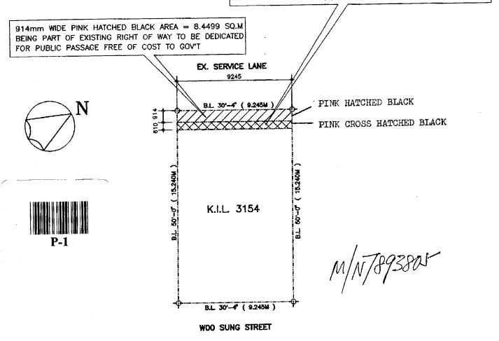
THE OWNER UNDERTAKERS TO PAY FOR THE COST FOR NECESSARY SURFACING, CHANNELLING, DRAINAGE WORKS AND ( IN APPROPRIATE CASE ) LIGHTING TO THE COLOURED PINK HATCHED BLACK AREA AND COLOURED PINK CROSS HATCHED BLACK AREA.
