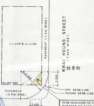
TO BE DEDICATED TO THE PUBLIC FOR THE PURPOSE OF PASSAGE AS REQUIRED BY HIGHWAYS DEPARTMENT. CORNER SPLAY AREA = 3.60 m2 & VERTICAL CLEARANCE OF 5.5 m. MIN.
