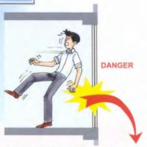
The unauthorized glass panels could not function as a safety barrier to prevent persons or objects from falling out.
