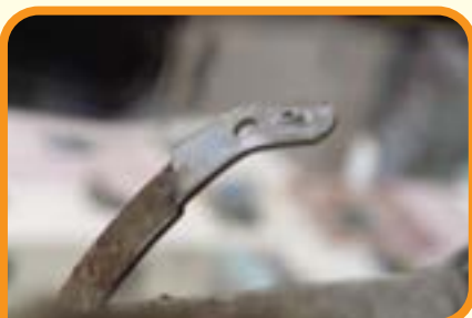
→ Bent or loose bar hinges
