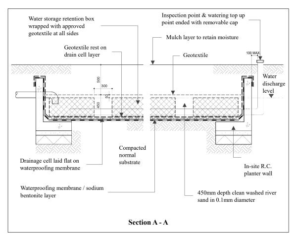
Diagram 4 – Sample of zero irrigation system (9/2023)
