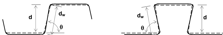
Figure 11.2b - Idealized section for sheet profile
