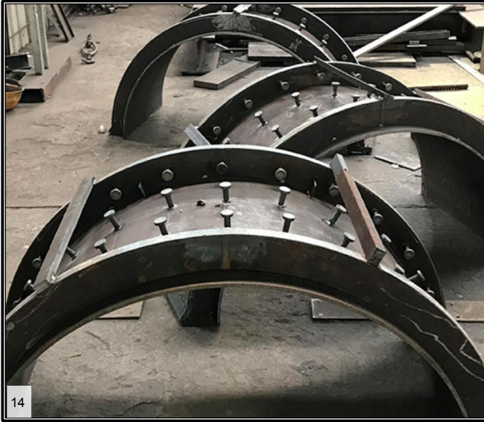
Plated steel arch to be installed under the existing arches (Source: Arup)
