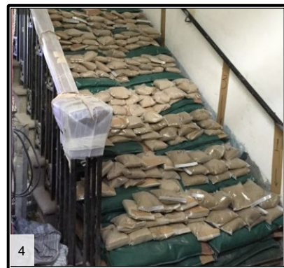
Proof load test of an existing granite staircase up to 1.25 times of the design load by using sand bags (Source: Arup)
