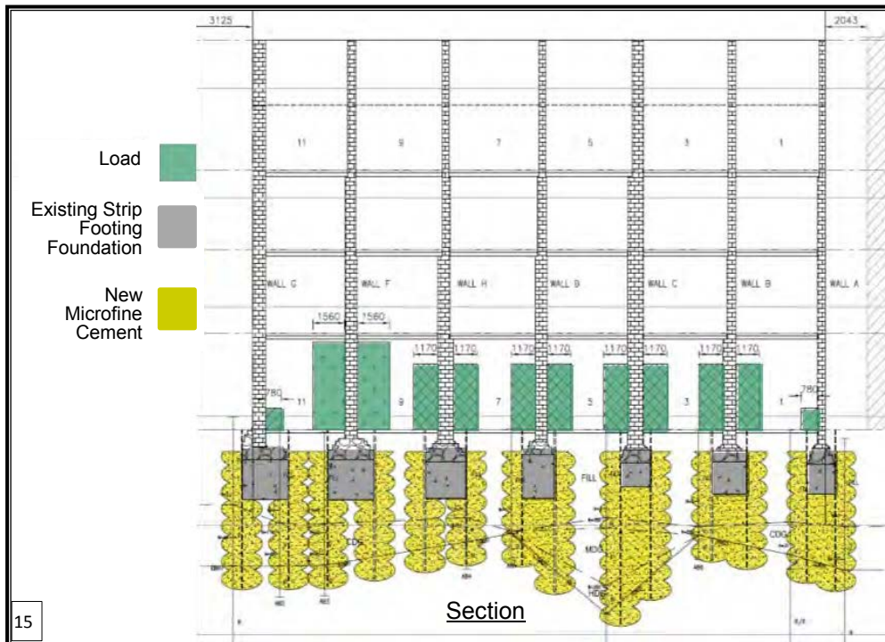
Strengthening of foundation by pressure grouting
