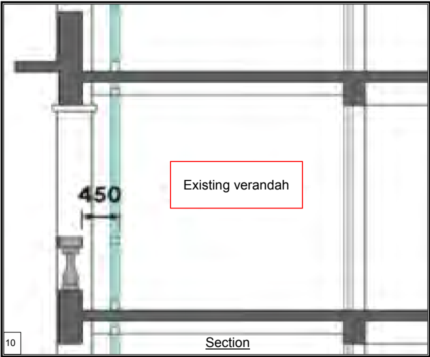
Setting out of tempered glass wall and existing balustrade
